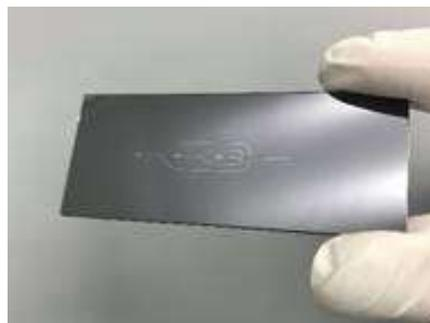
***Silicon chips and etched microfluidic channels with hermetically bonded glass cap***
