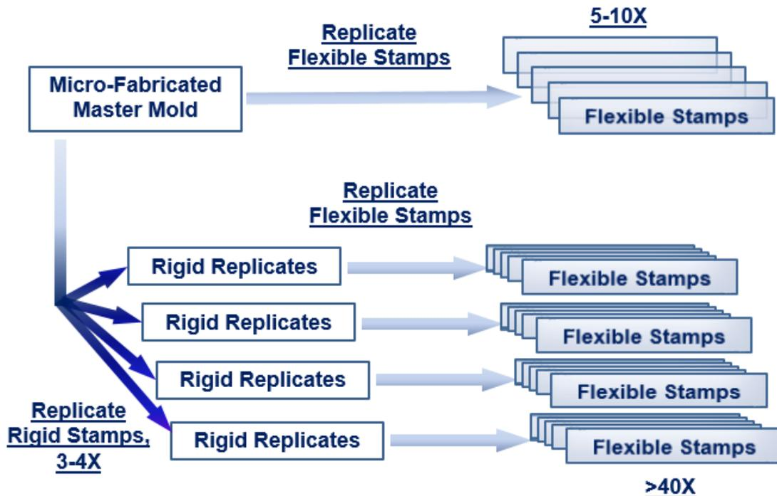
**Figure 4: Typical pathways to produce multiple flexible stamps from a micro-fabricated master mold for micro-fluidic devices.**
