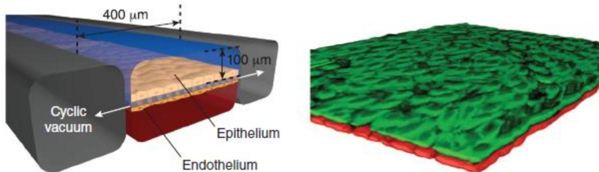
**Figure 2:** A schematic view of the 'breathing' lung-on-a-chip that recapitulates the alveoli-capillary interface (Left) and the fluorescence confocal 3D reconstruction (Right). [4]
