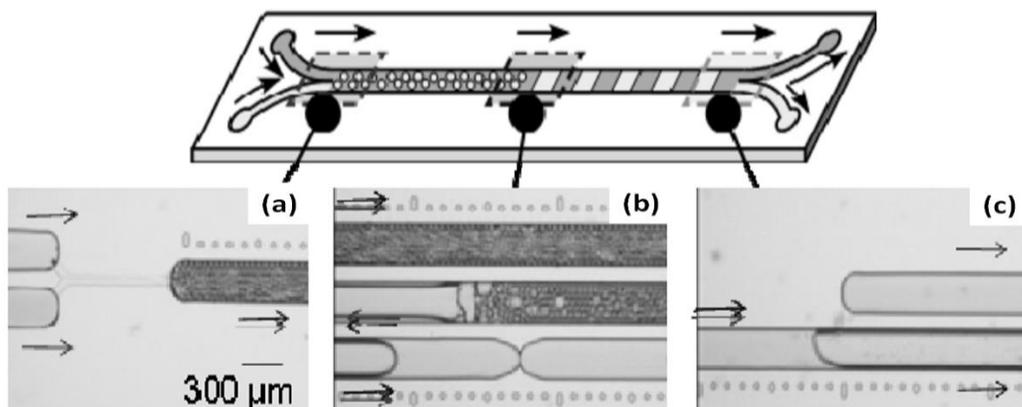
**Figure 1: Demonstration of in-flow (a) droplet formation, (b) droplet-to-plug conversion and (c) separation of two-phase liquid by controlling surface chemistry of micro-channels. [3]**
