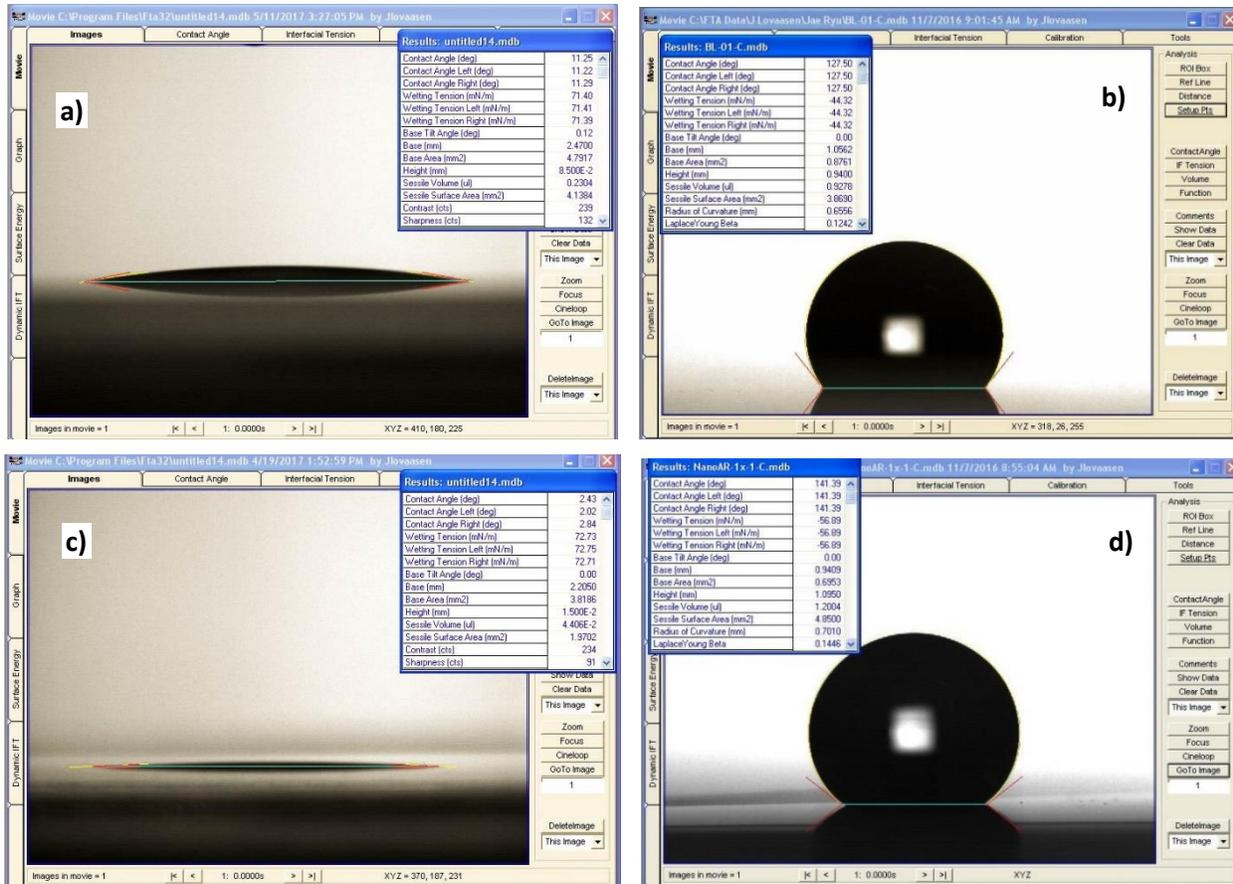
**Figure 3:** Various bio-compatible materials which are used for micro-biomedical systems: (a) inherently hydrophilic glass wafer; (b) inherently hydrophobic glass wafer; (c) super-hydrophilic plasma treated glass; and (d) super-hydrophobic nano-textured surface.
