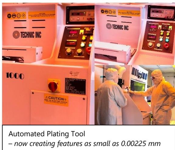
The electroplating cell is able to plate and electroform wafers or discreet parts up to a size of 200 mm (8"). Typical applications of this capability include MEMS, integrated circuits on silicon, gallium arsenide and similar glass-type substrates. Sensera's qualified processes on this cell achieve exceptionally low residual stress and enable tight thickness uniformity control.
